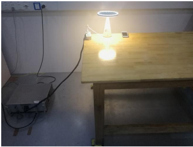
Conducted Emissions Test Setup Front View
