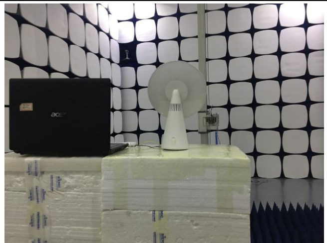
Radiated Spurious Emissions Test Setup Above 1GHz
