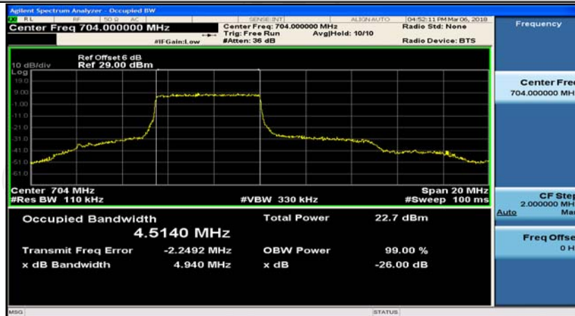
Channel Bandwidth: 10 MHz_LCH_QPSK_25RB#12
