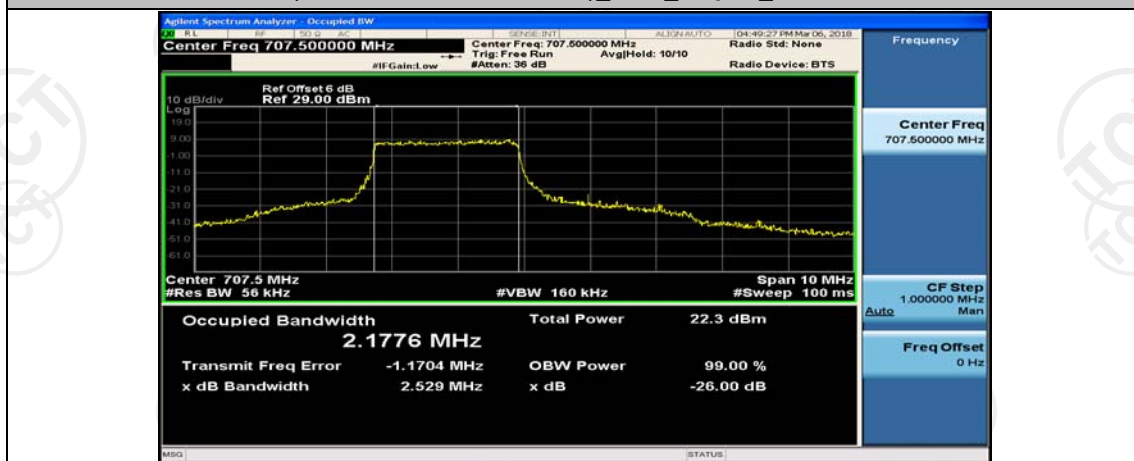
(Channel Bandwidth: 5 MHz)_MCH_16QAM_12RB#6
