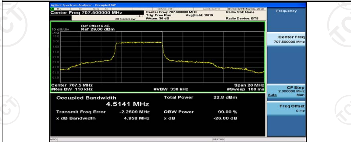
Channel Bandwidth: 10 MHz_MCH_QPSK_25RB#12
