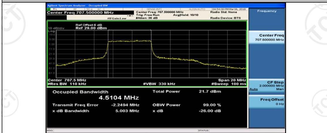
Channel Bandwidth: 10 MHz_MCH_16QAM_25RB#12
