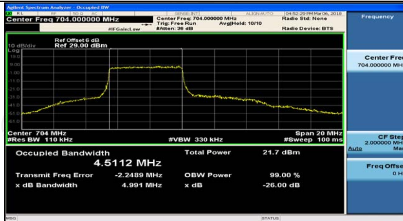
Channel Bandwidth: 10 MHz_LCH_16QAM_25RB#12
