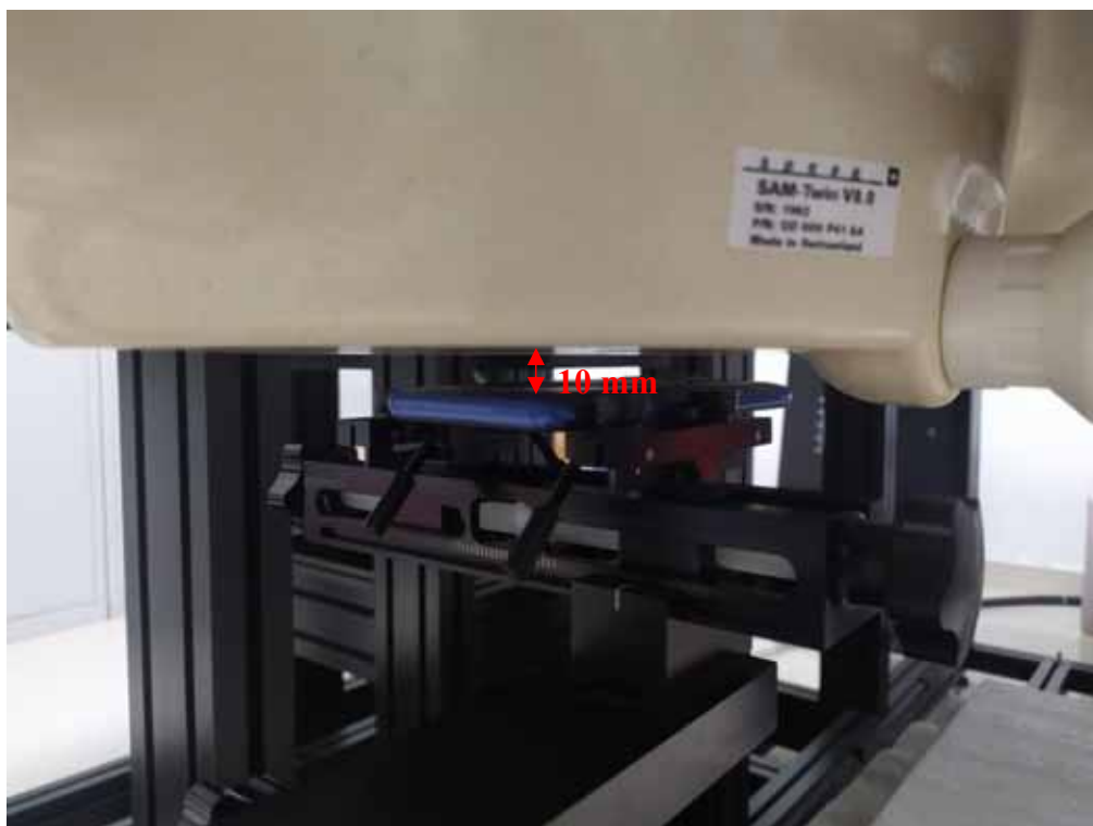
Body (Worn) Back Setup Photo (10mm)
