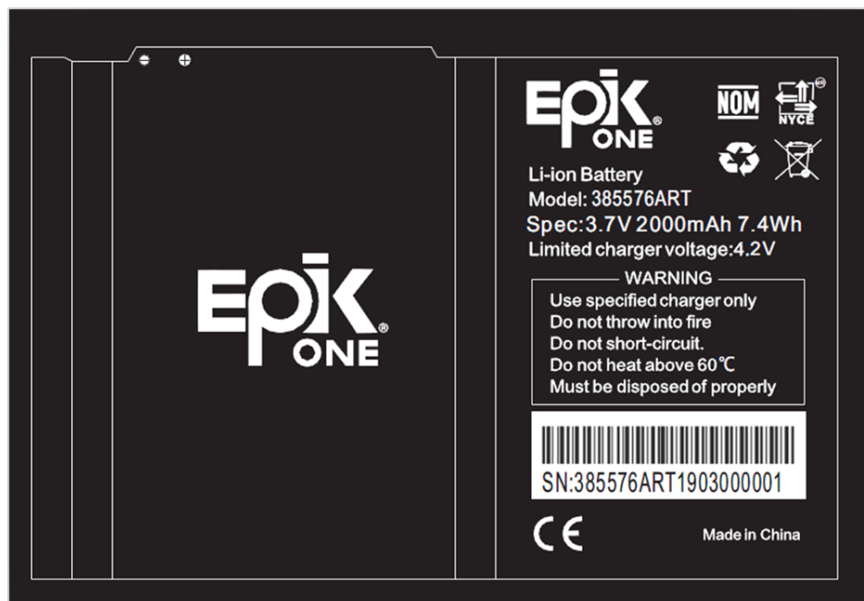
EUT – Battery Label View
