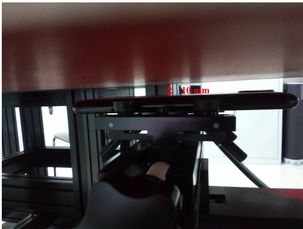
Body (Worn) Back Setup Photo (10mm)
