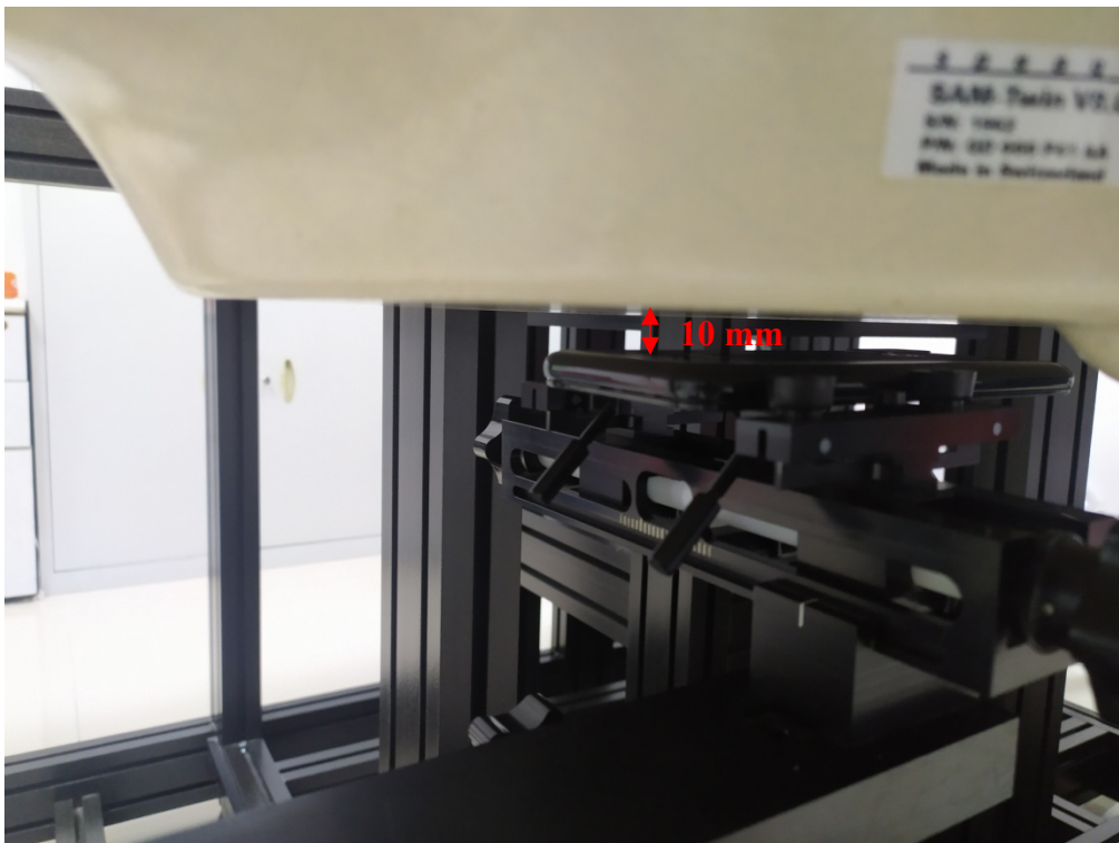
Body (Worn) Back Setup Photo (10mm)
