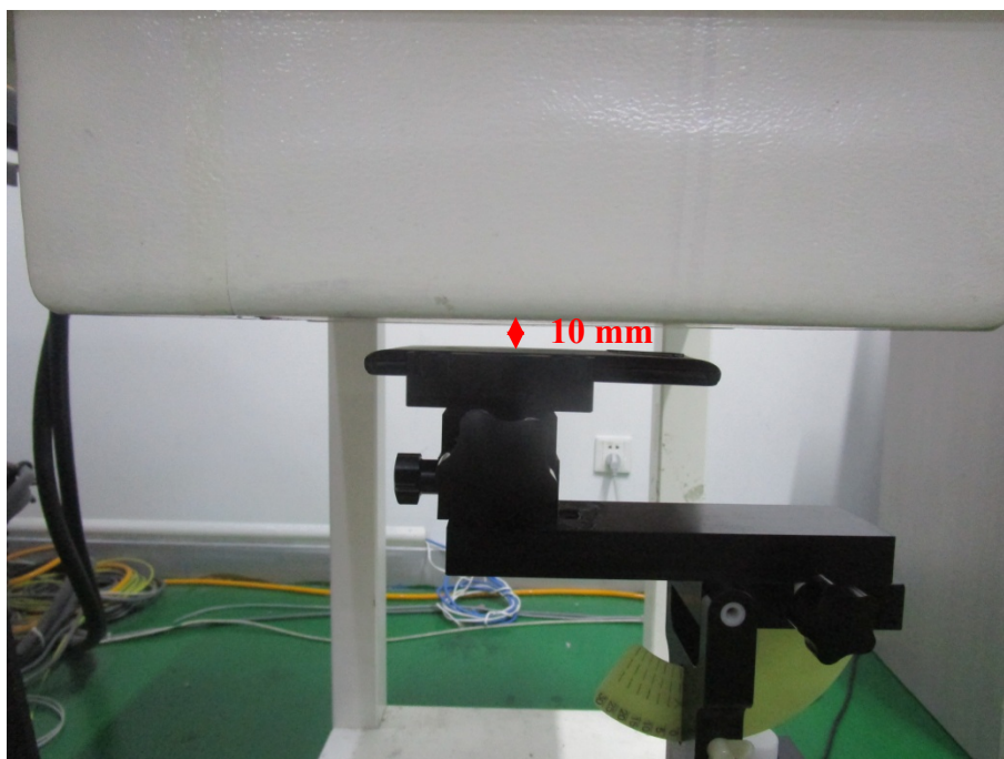
Body Right Setup Photo(10mm)
