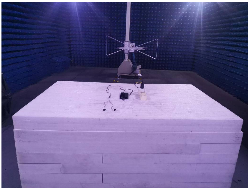
Photo of Radiated Emission Measurement (Below 1G)
