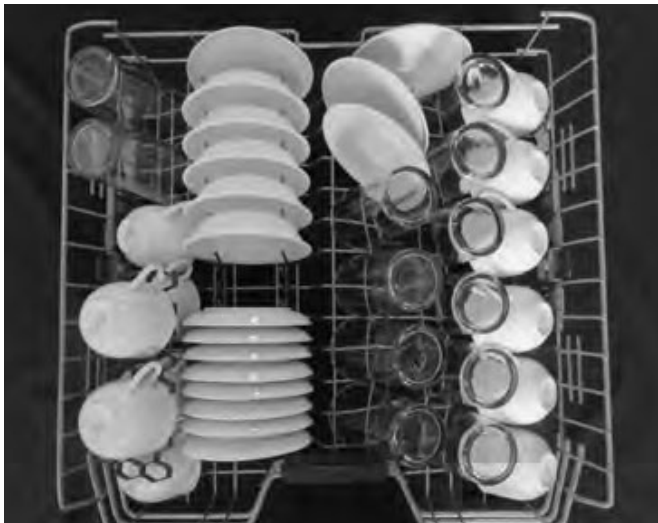
Top rack load pattern for 12 place settings according to the AHAM DW-1 Standards
