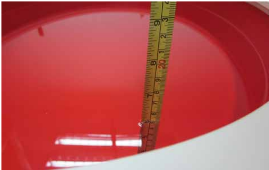
Figure 4.4: Liquid depth in the Flat Phantom
