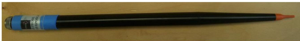
Figure 1 – MVG COMOSAR Dosimetric E field Dipole
