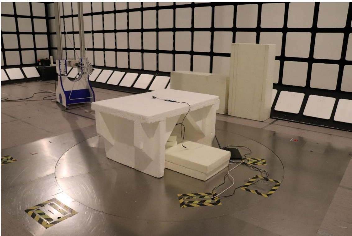
Photograph 2. Test Setup for Radiated Emissions 30 – 1000 MHz
