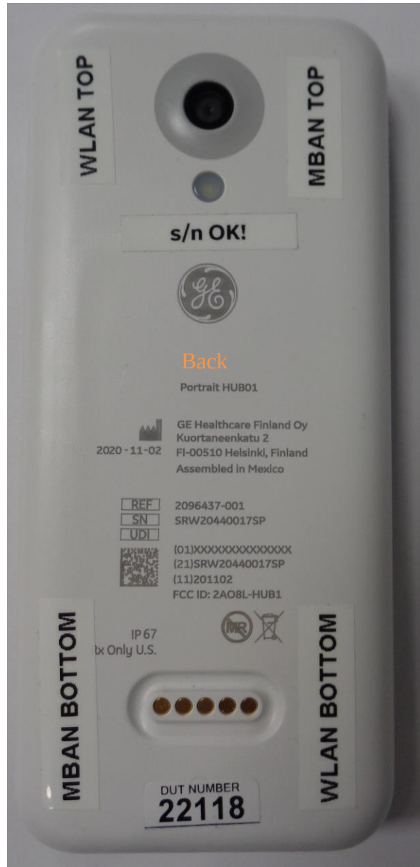
Back side of the HUB and antenna locations
