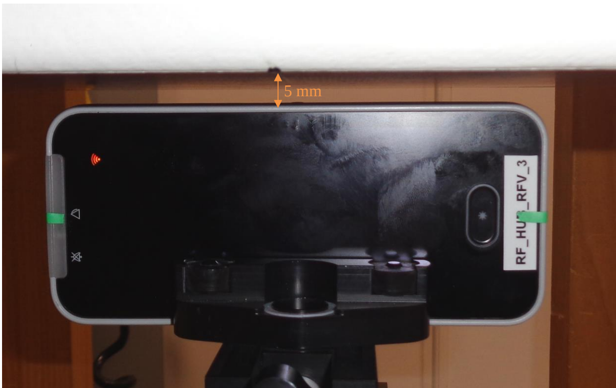
Right side of the HUB against the phantom, 5mm separation distance
