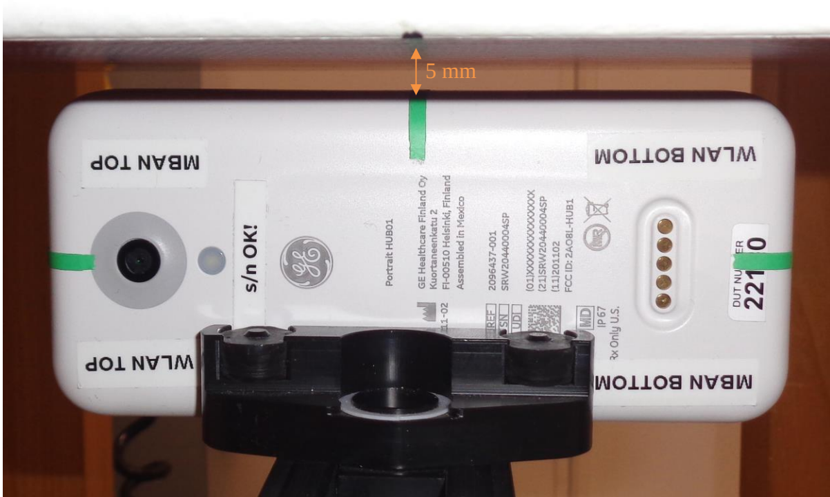
Left side of the HUB against the phantom, 5mm separation distance
