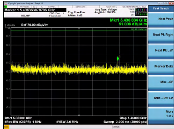
5350-5460 MHz, Channel 48, MCS0, Peak Vertical Antenna
