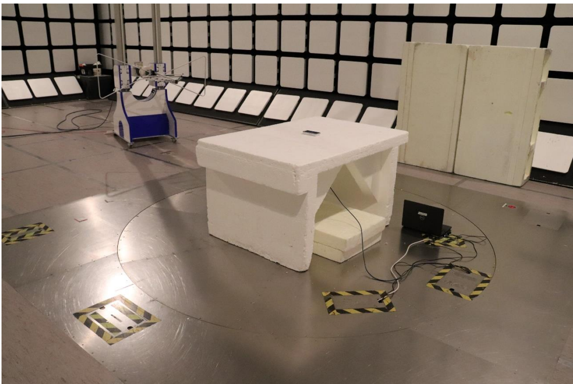
Photograph 2. Test Setup for Radiated Emissions 30 – 1000 MHz
