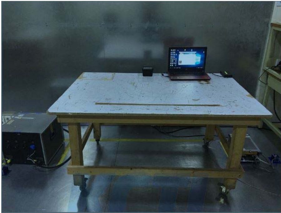
Conducted Emission Setup Photo
