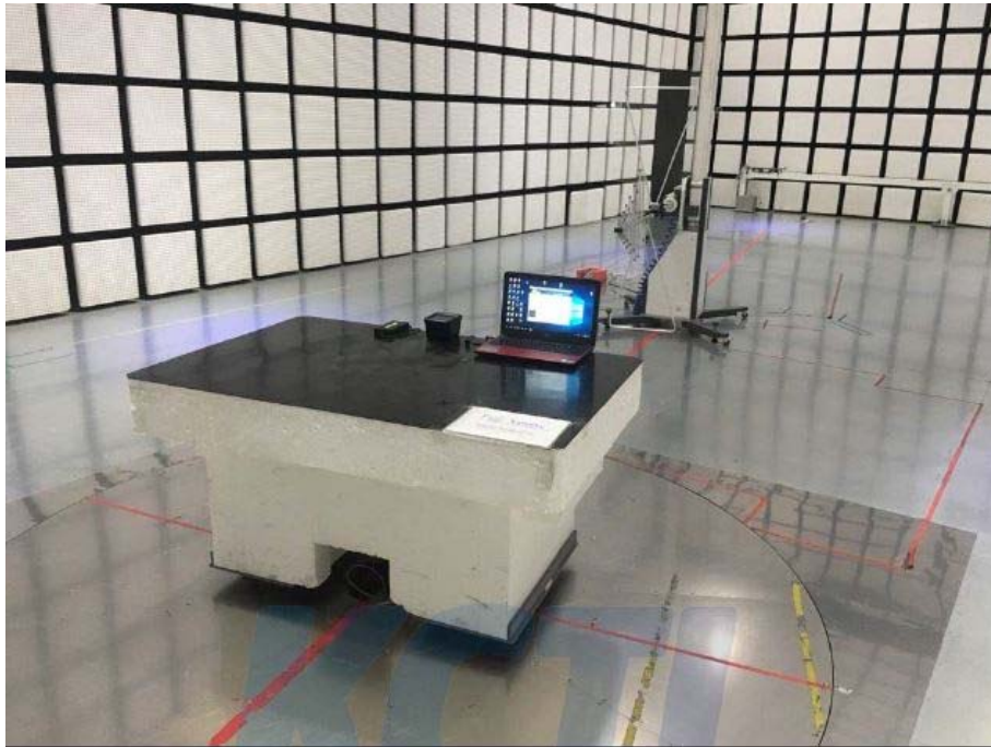
Radiated Emission Setup photo
