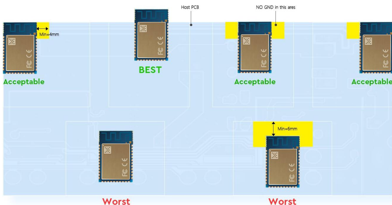
Figure 7: Recommended Module Mounting Examples
