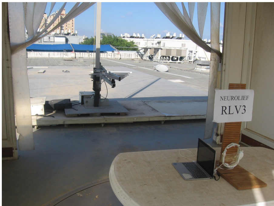
Figure 6. Radiated Emission Test, 200-1000MHz
