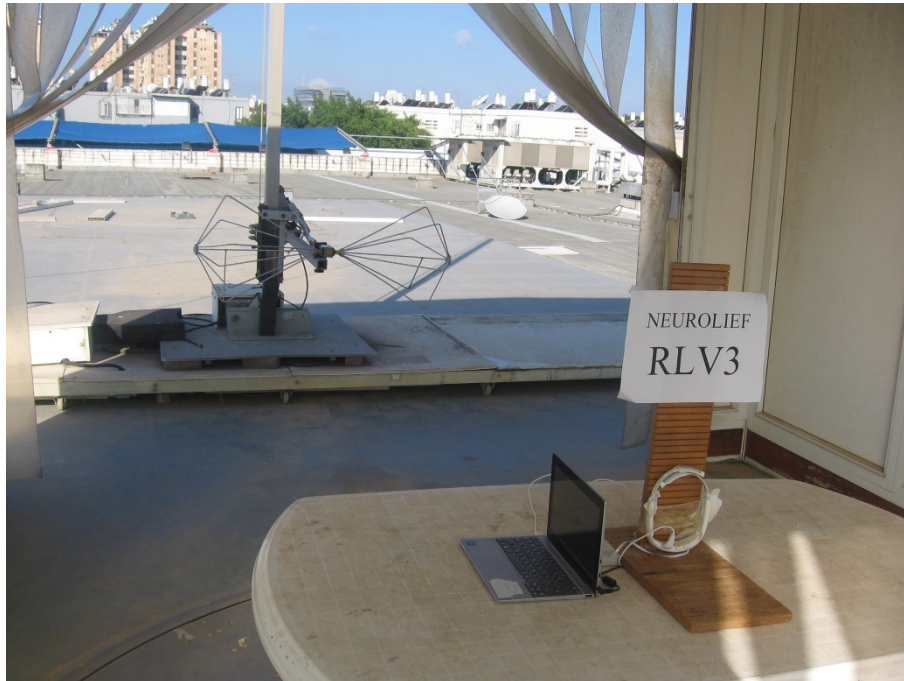
Figure 5. Radiated Emission Test, 30-200MHz
