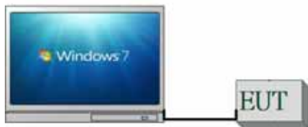
Fig. 2-2 Conducted (Antenna Port) Emission Configuration
