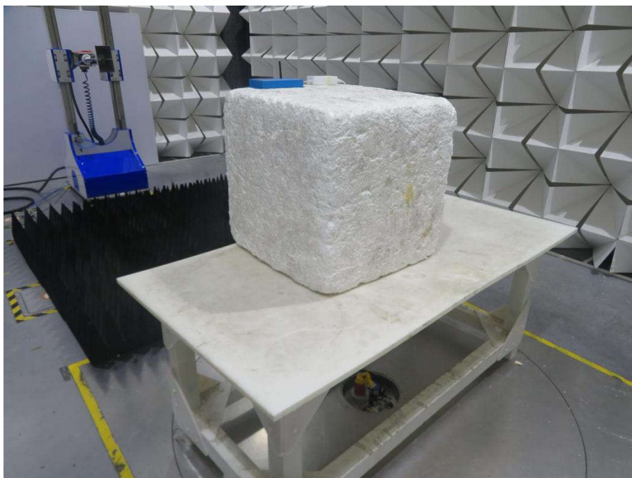
Radiated spurious emission Test Setup-3(Above 1GHz)
