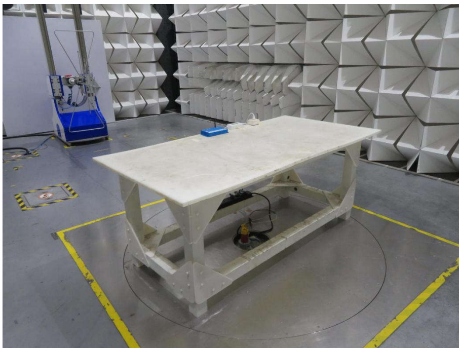
Radiated spurious emission Test Setup-2(30MHz-1GHz)
