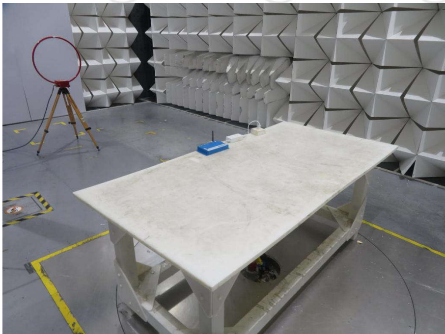
Radiated spurious emission Test Setup-1(Below 30MHz)
