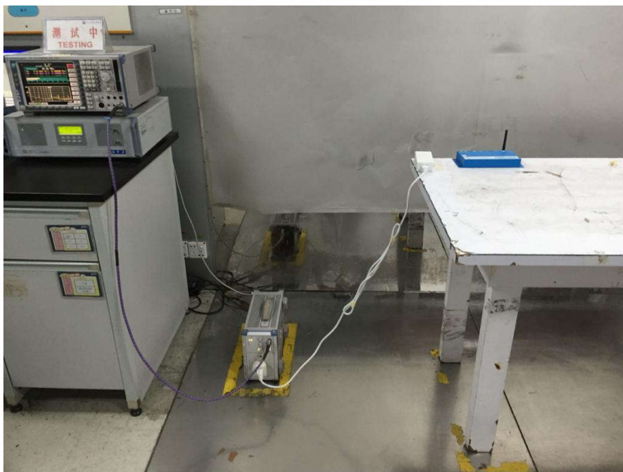
Conducted Emissions Test Setup
