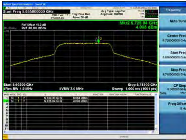
Peak Power Spectral Density Data Plot (CH High 5720 MHz)
