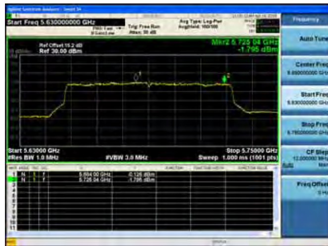
802.11ac VHT80, 5725~5850 MHz Peak Power Spectral Density Data Plot (CH Mid 5775 MHz)
