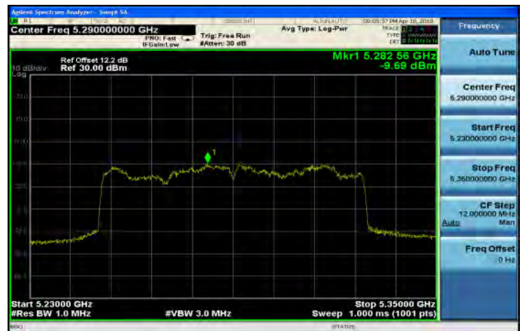
Peak Power Spectral Density Data Plot (CH Mid 5290 MHz)
