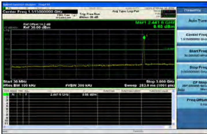
802.11g: Spurious Emission Test Data CH-Mid
