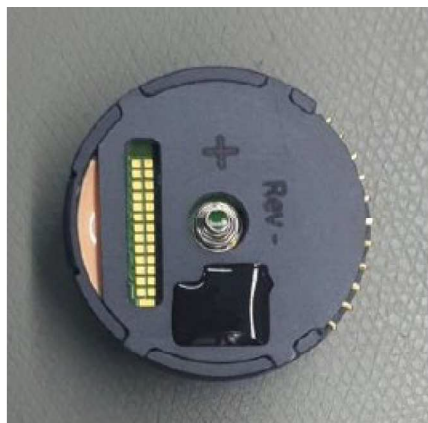
Figure 1 Circuit Boards Permanently Set in Encapsulant
