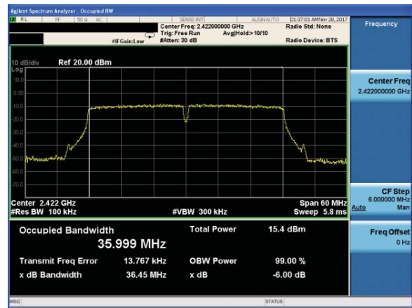
(802.11n40) 6dB Bandwidth plot on channel 6
