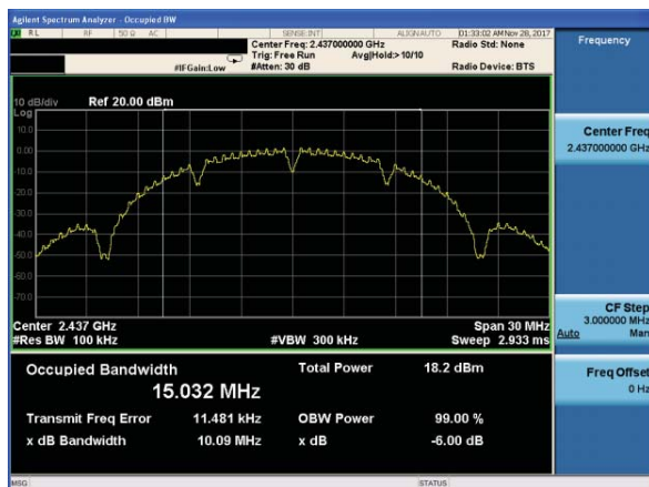
(802.11b) 6dB Bandwidth plot on channel 6
