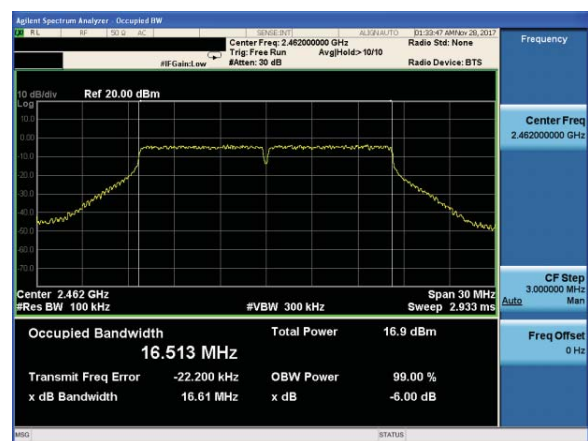
(802.11g) 6dB Bandwidth plot on channel 11
