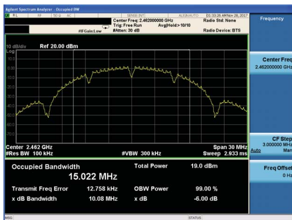
(802.11b) 6dB Bandwidth plot on channel 11
