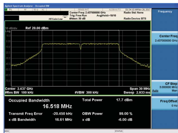
(802.11g) 6dB Bandwidth plot on channel 6
