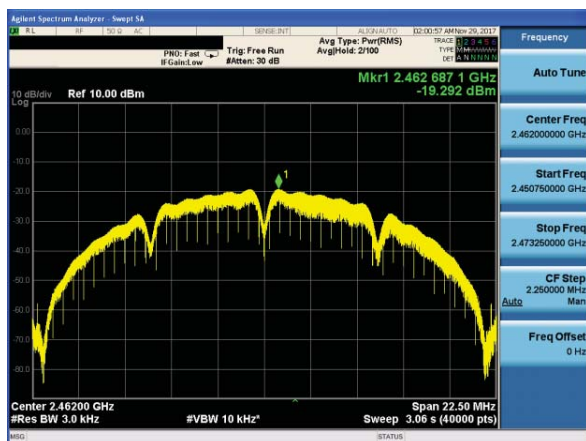
(802.11b) PSD plot on channel 11
