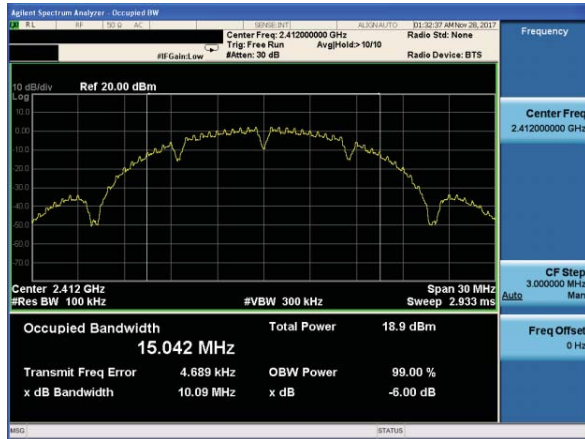
(802.11b) 6dB Bandwidth plot on channel 6
