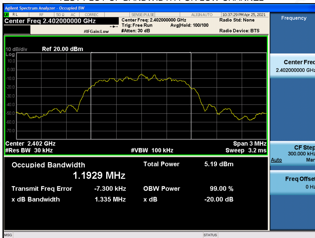
TEST PLOT OF BANDWIDTH FOR LOW CHANNEL
