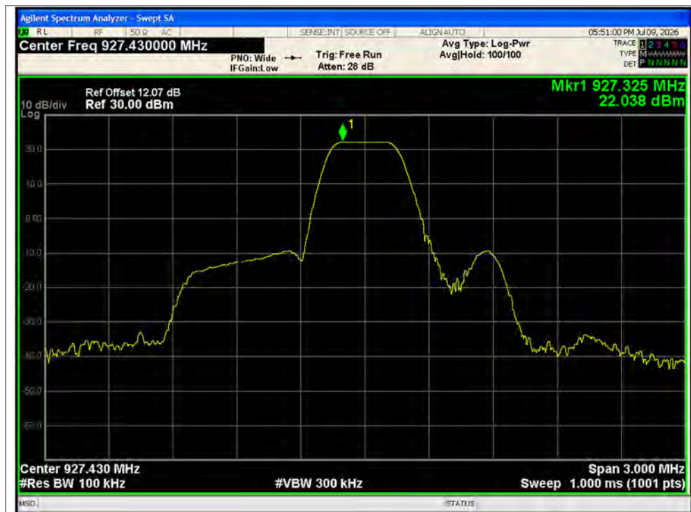
Band Edge NVNT LoRa 927.43MHz Ant1 No-Hopping Ref
