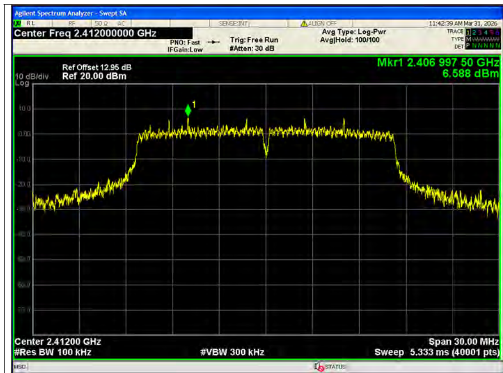
Tx. Spurious NVNT g 2412MHz Ant2 Ref
