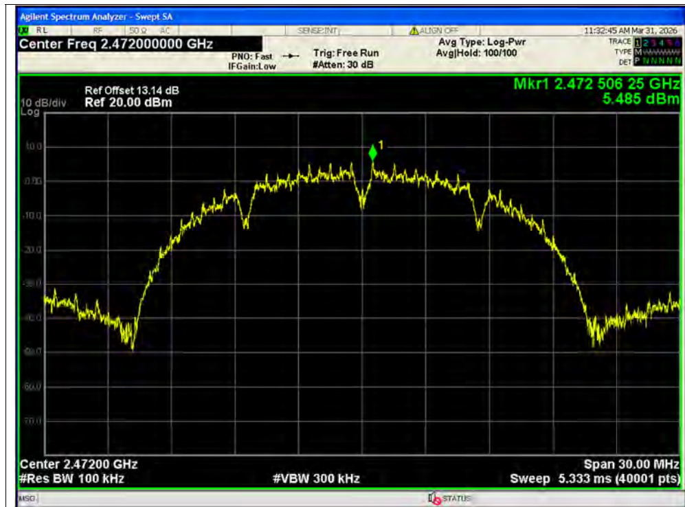
Tx. Spurious NVNT b 2472MHz Ant2 Ref
