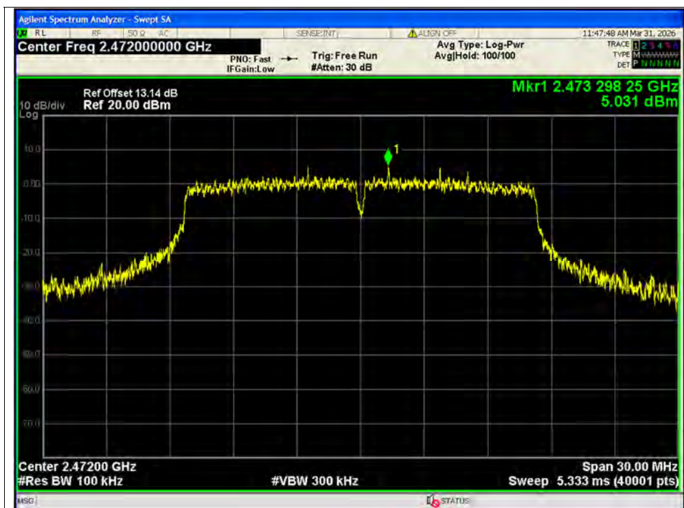
Tx. Spurious NVNT g 2472MHz Ant2 Ref
