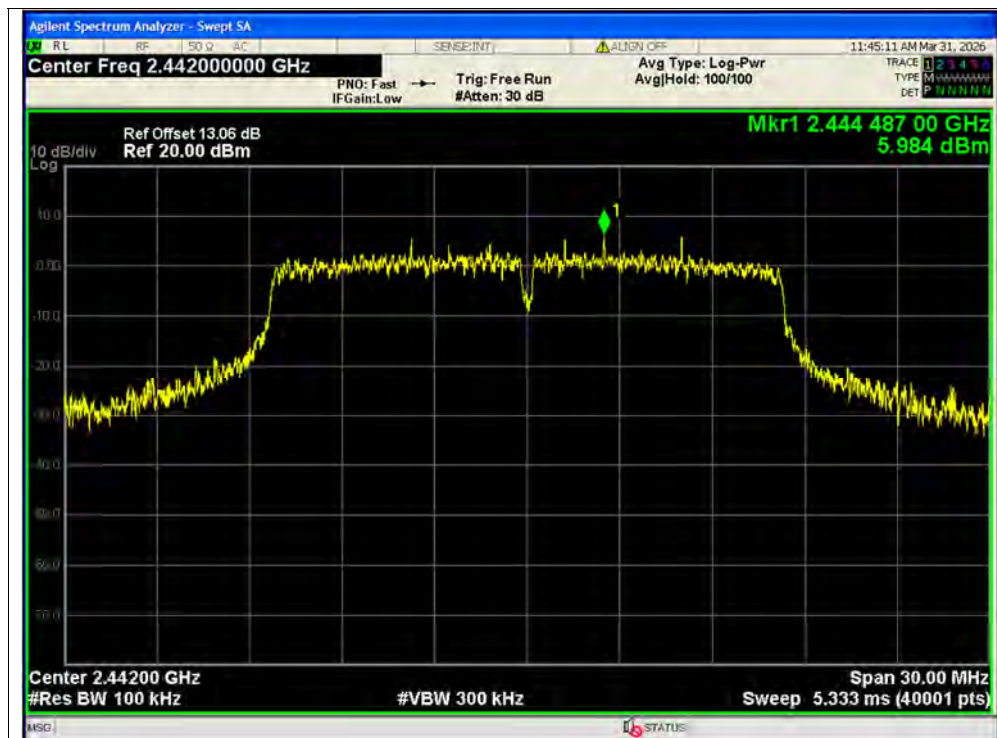
Tx. Spurious NVNT g 2442MHz Ant2 Ref
