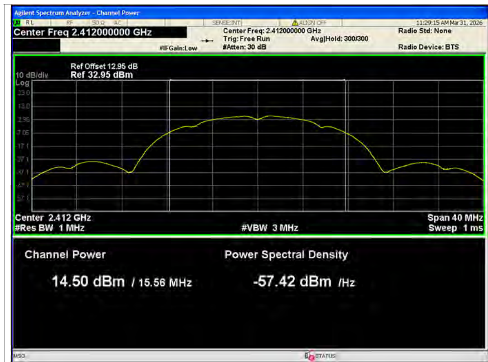
Average Power NVNT b 2412MHz Ant2
