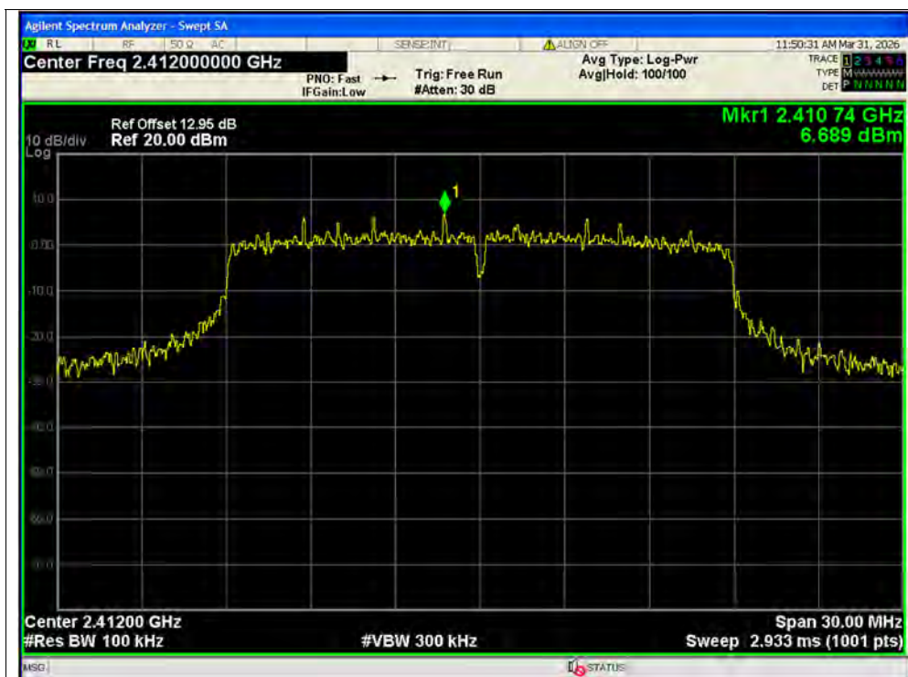
Band Edge NVNT n20 2412MHz Ant2 Ref
