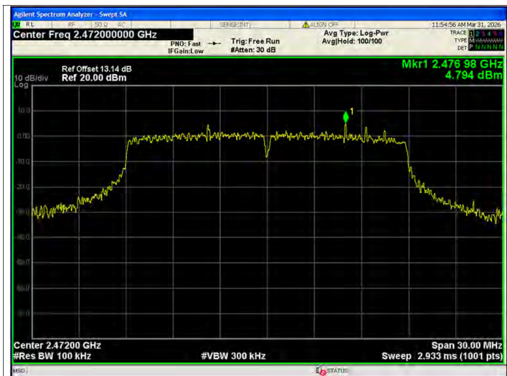
Band Edge NVNT n20 2472MHz Ant2 Ref
