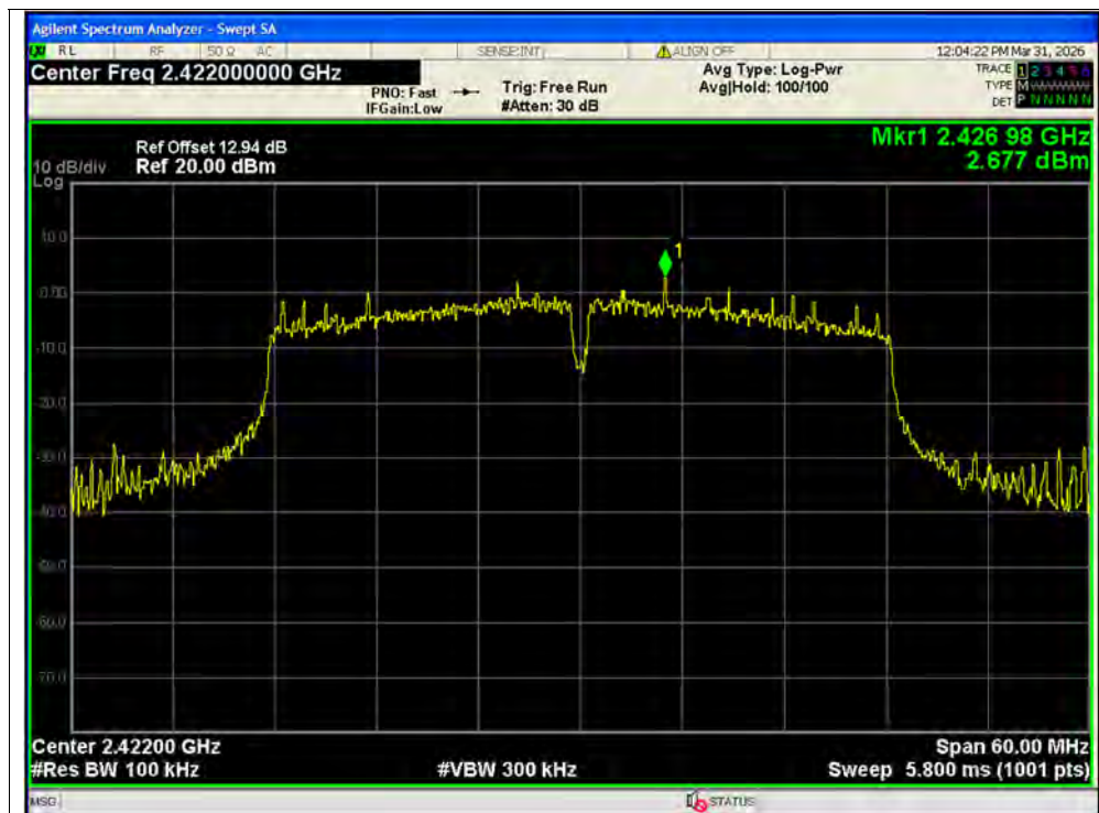
Band Edge NVNT n40 2422MHz Ant2 Ref
