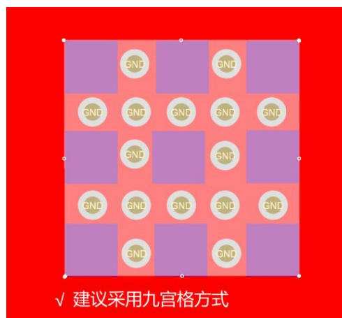
Figure 4.4 The nine-square grid method of the floor EXPAD
