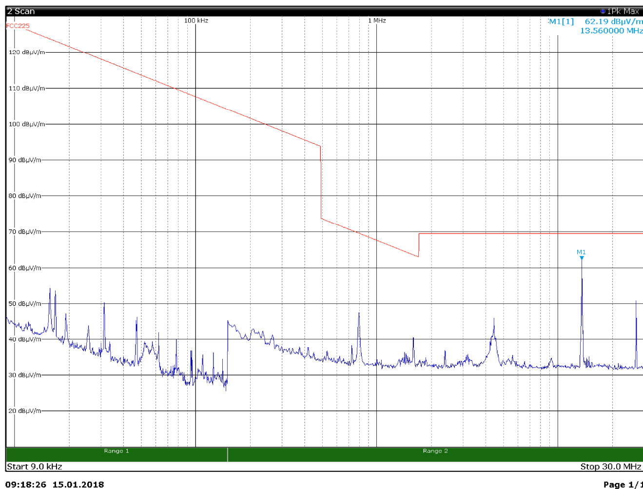
Figure 8.3-1: Field strength of spurious emissions below 30 MHz
