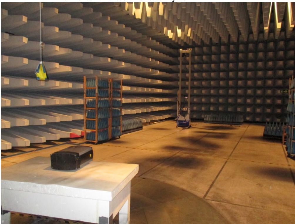
Photo 4.1.4 Test setup regarding measurement of radio frequency electromagnetic field. Horizontal orientation of test object
