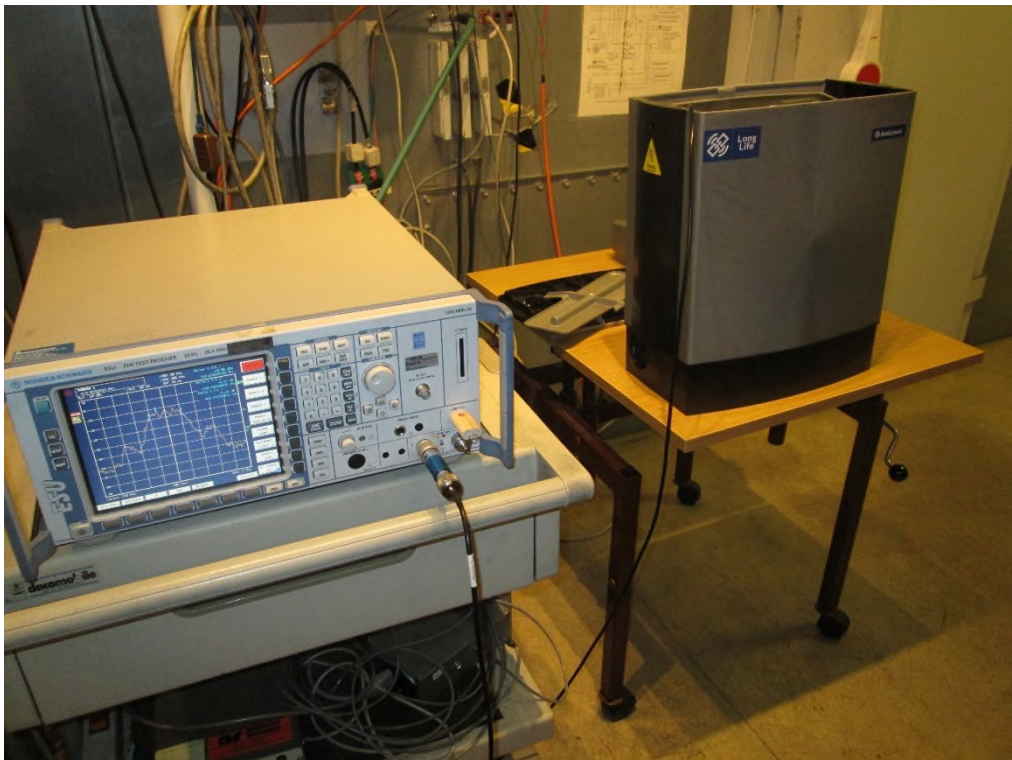
Photo 4.4.2 Test setup regarding measurement of 6 dB bandwidth.
