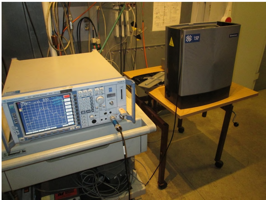
Photo 4.5.2 Test setup regarding measurement of 20 dB bandwidth.
