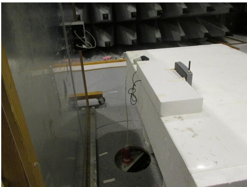
Photo 4.7.2 Test setup regarding measurement of radio frequency voltage on mains.
