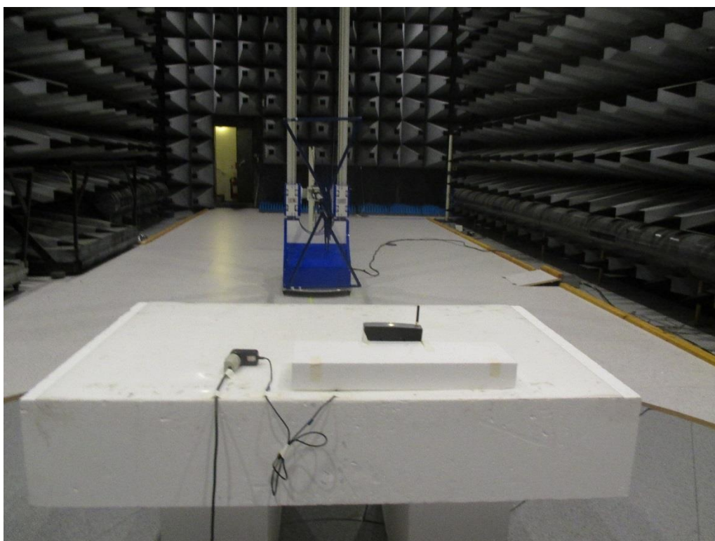
Photo 4.8.2 Test setup regarding measurement of radiated emission (below 1 GHz).
