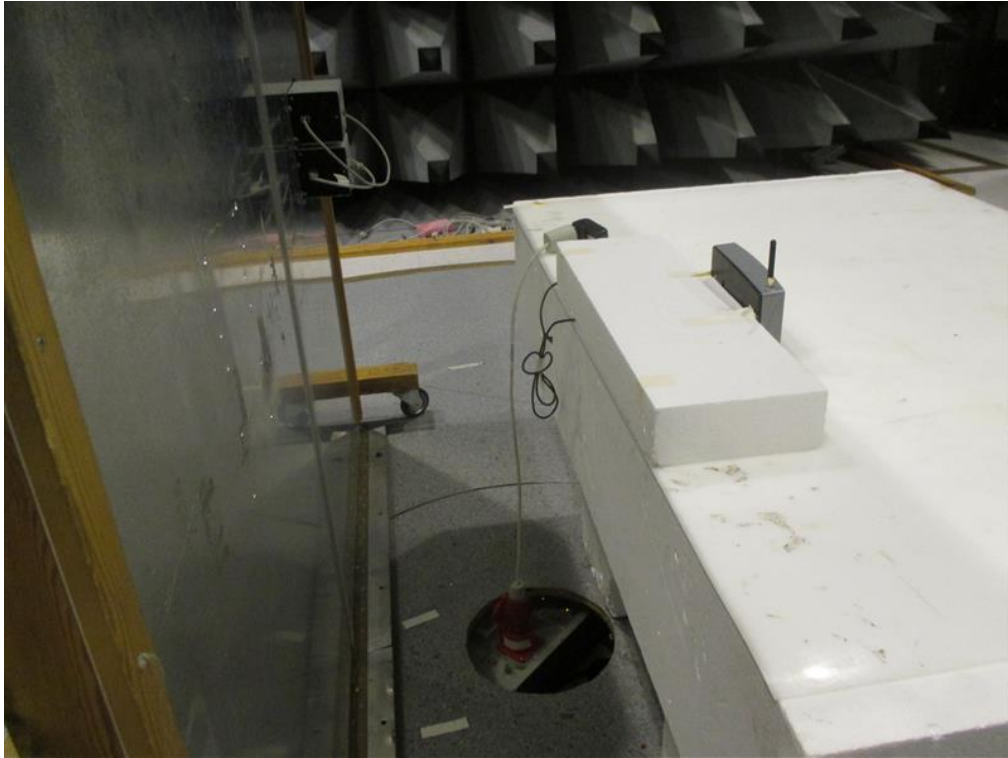
Photo 4.1.2 Test setup regarding measurement of radio frequency voltage on mains.
