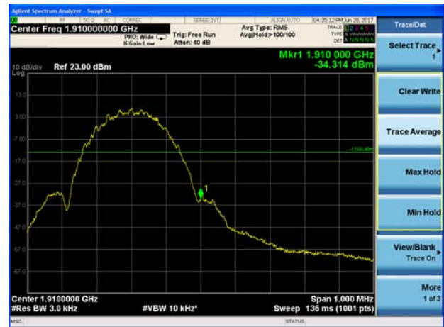
LTE Band 2 1.4MHz QPSK 1RB CH-High
