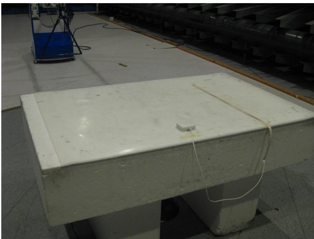
Photo 4.8.2 Test set-up regarding measurement of radiated emission (below 1 GHz).
