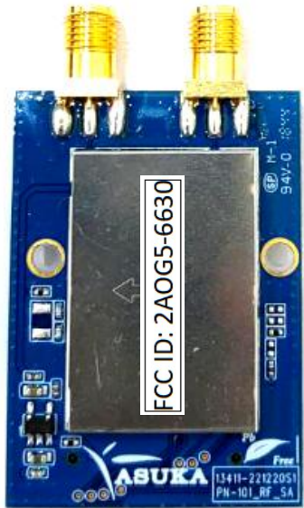
WiFi/BT/GPS RF Module Model Name: AK-6630
