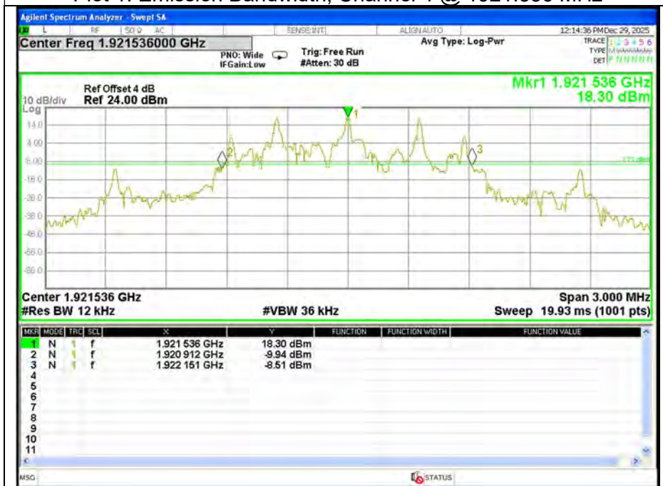
Plot 1. Emission Bandwidth, Channel 4 @ 1921.536 MHz
