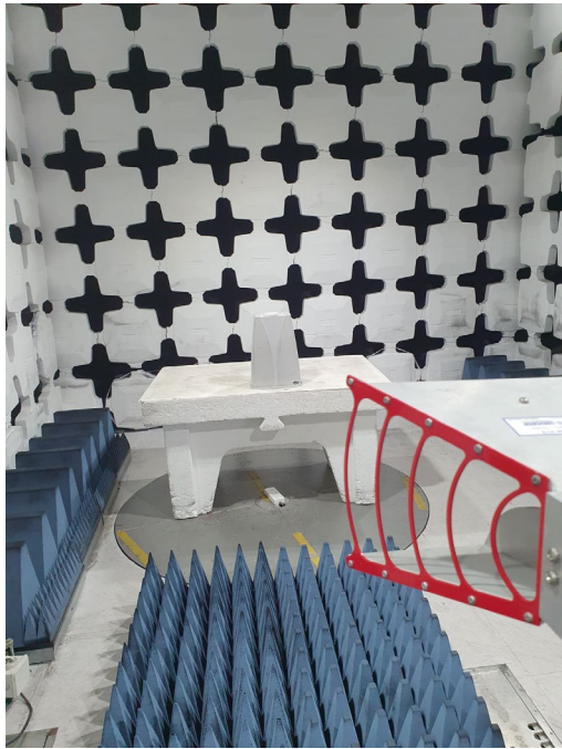
Radiated emissions test set up above 1GHz.
