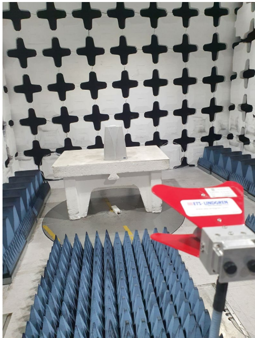
Radiated emissions test set up above 18GHz.
