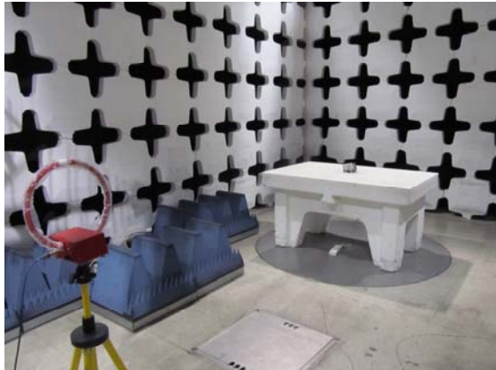
Radiated emissions test set up below 30MHz.
