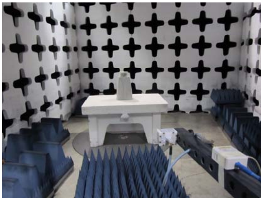
Radiated emissions test set up above 18GHz.
