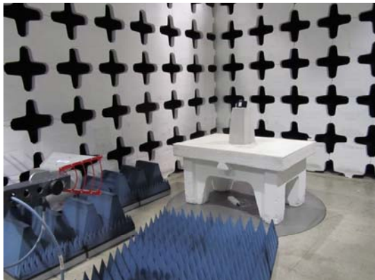
Radiated emissions test set up above 1GHz.
