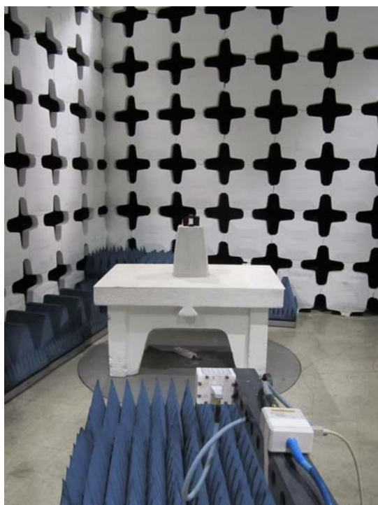
Radiated emissions test set up above 18GHz.
