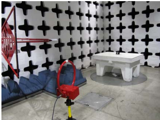
Radiated emissions test set up below 30MHz.
