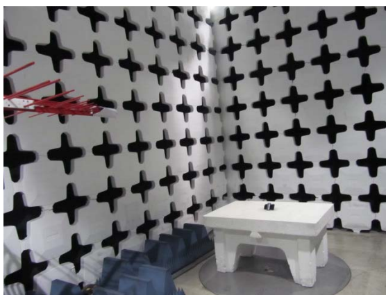
Radiated emissions test set up below 30MHz.
