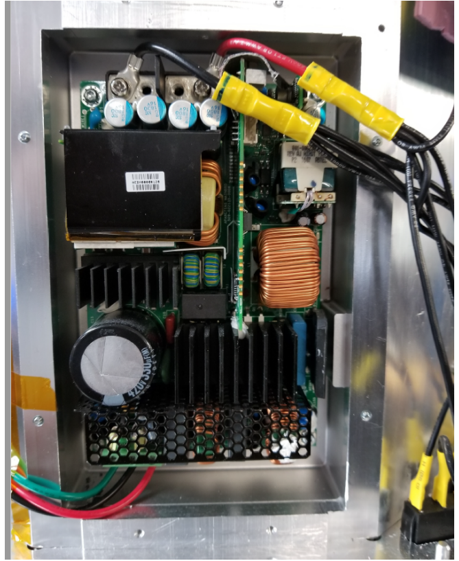
AC Power Supply Unit
