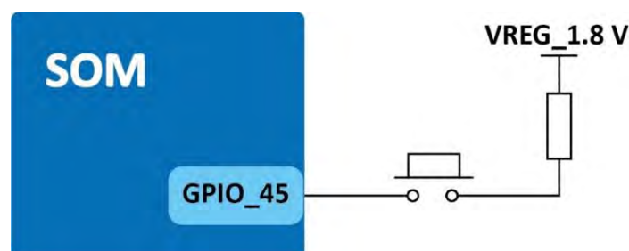
Figure 2-4. Power on Signal
