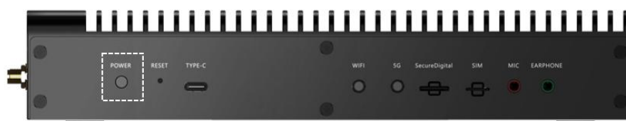
Figure 4-2. Power Button/instructor location instruction
