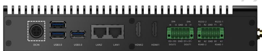
Figure 4-1. Power connector location instruction
