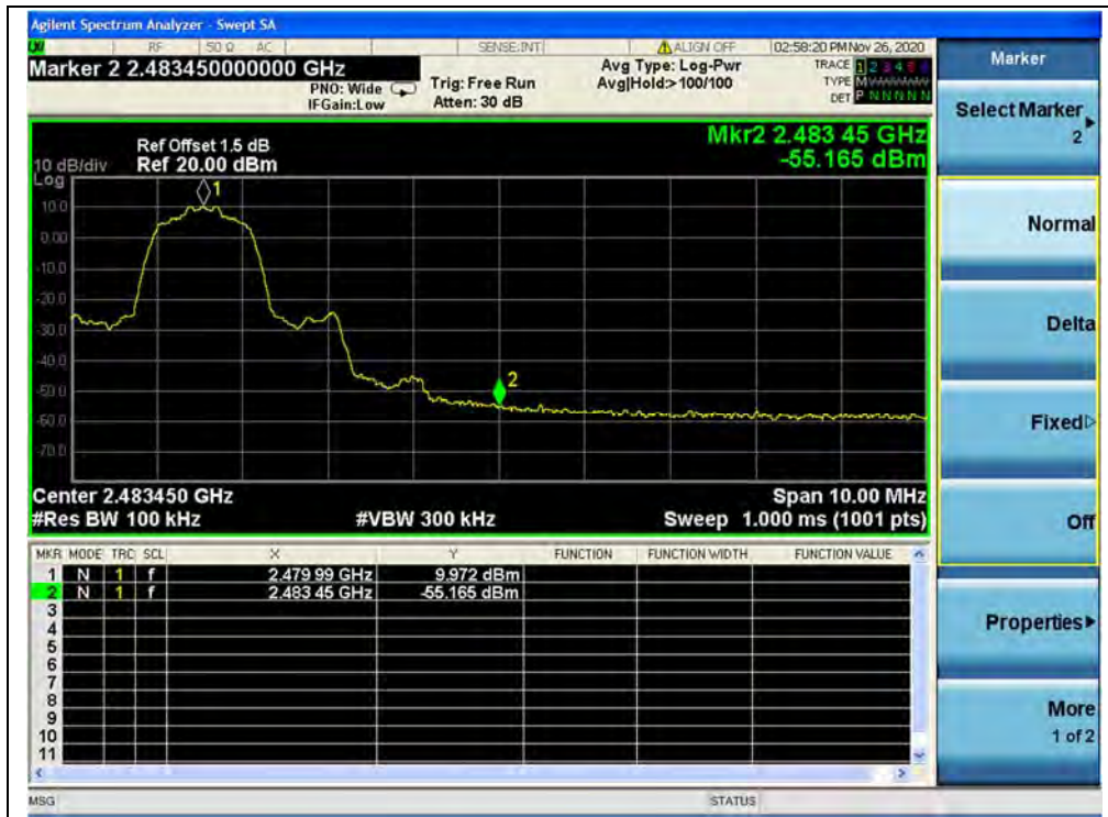
(Band edge, Channel 78, \pi/4 -DQPSK)
