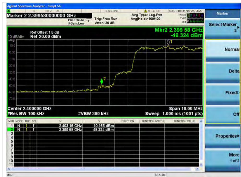
(Band edge with hopping on, Channel 0, 8-DPSK)
