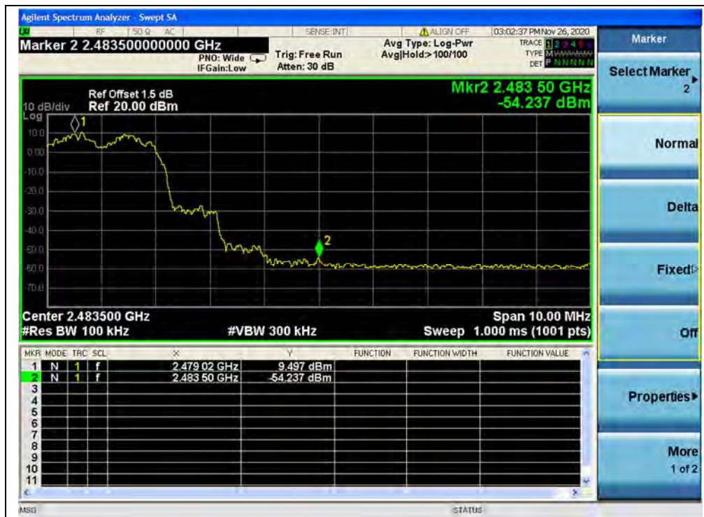
(Band edge with hopping on, Channel 78, 8-DPSK)
