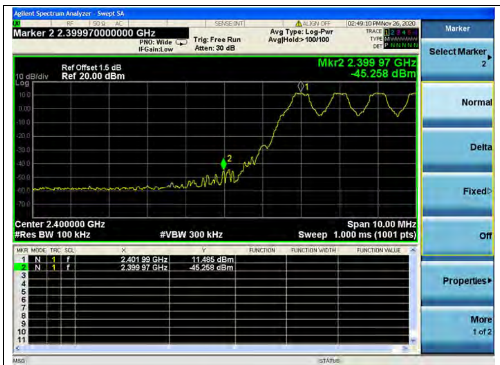
(Band edge with hopping on, Channel 0, GFSK)
