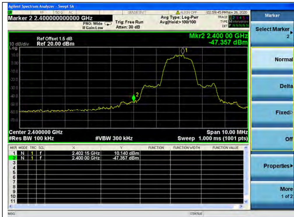
(Band edge, Channel 0, \pi/4 -DQPSK)
