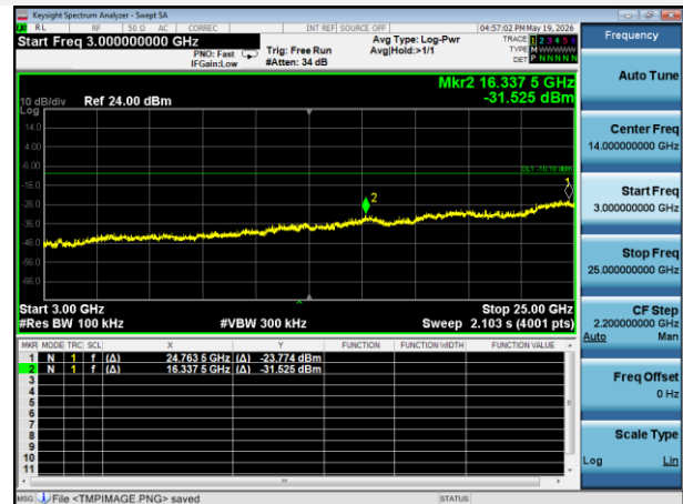
GFSK LOW CHANNEL, SPURIOUS 3 GHz ~ 25 GHz
