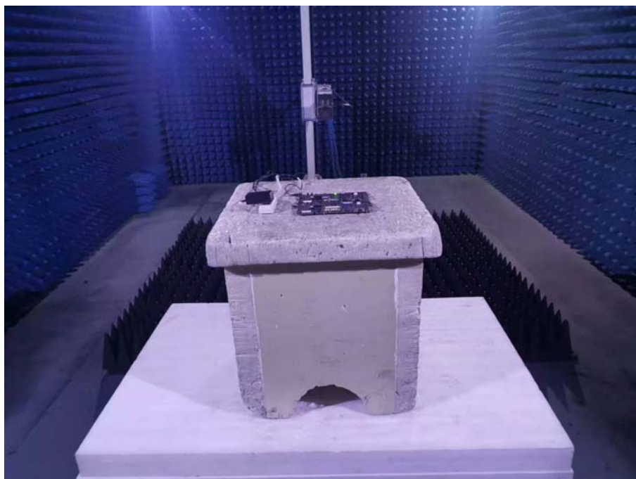
Photo of Radiated Emission Measurement (Above 1G)
