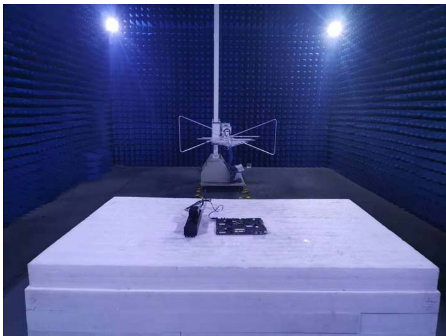
Photo of Radiated Emission Measurement (Above 1G)
