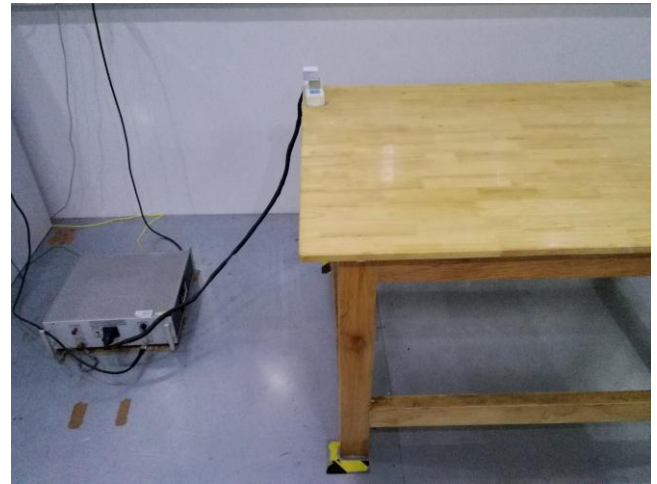
Conducted Emissions Test Setup Side View
