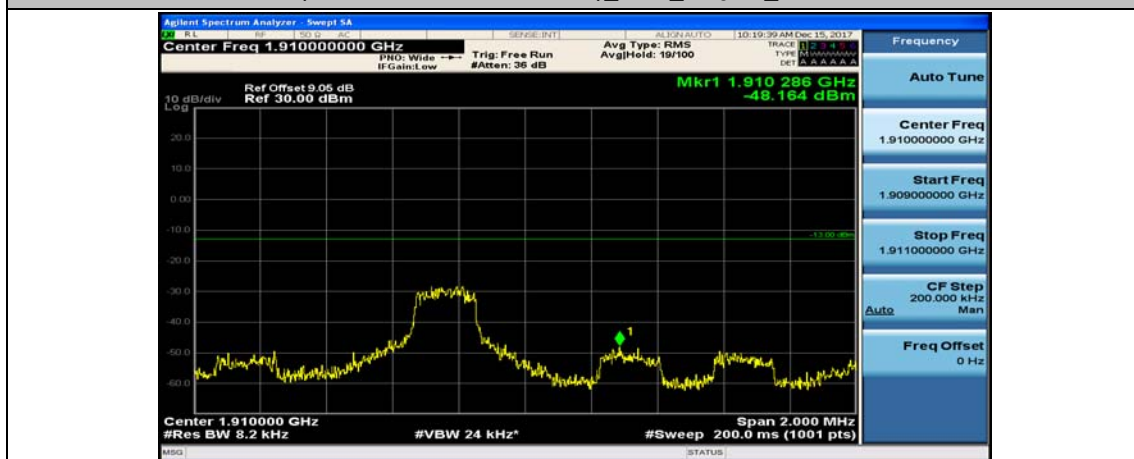
(Channel Bandwidth: 3 MHz)_HCH_16QAM_1RB#7
