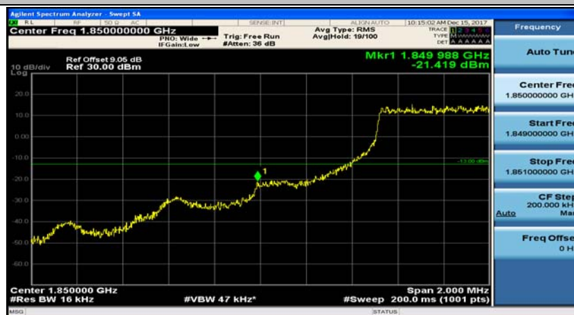
(Channel Bandwidth: 1.4 MHz)_LCH_QPSK_3RB#3
