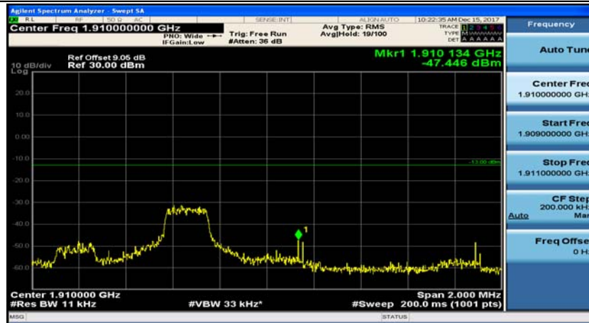
(Channel Bandwidth: 5 MHz)_HCH_QPSK_1RB#12
