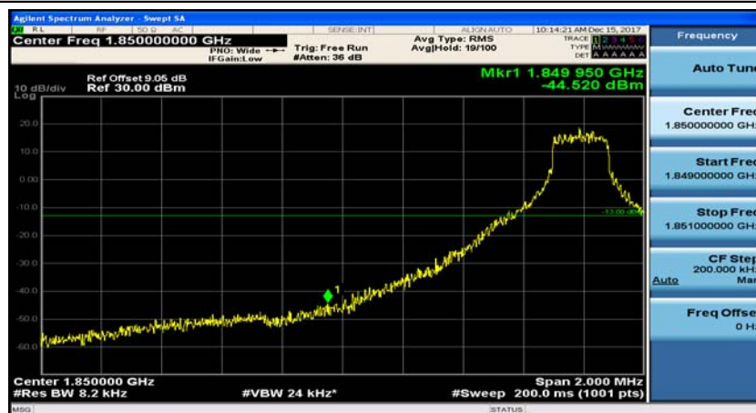
(Channel Bandwidth: 1.4 MHz)_LCH_QPSK_1RB#5
