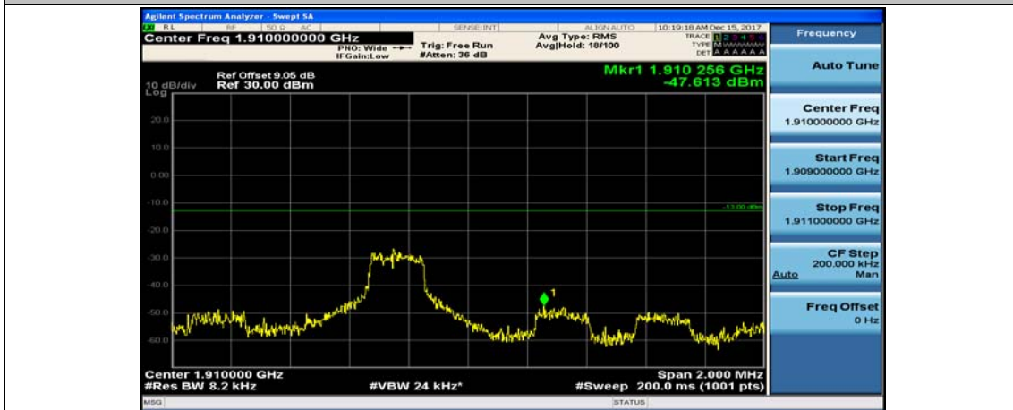
(Channel Bandwidth: 3 MHz)_HCH_QPSK_1RB#7
