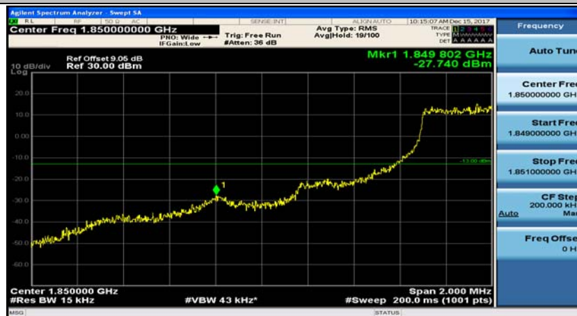
(Channel Bandwidth: 1.4 MHz)_LCH_QPSK_6RB#0
