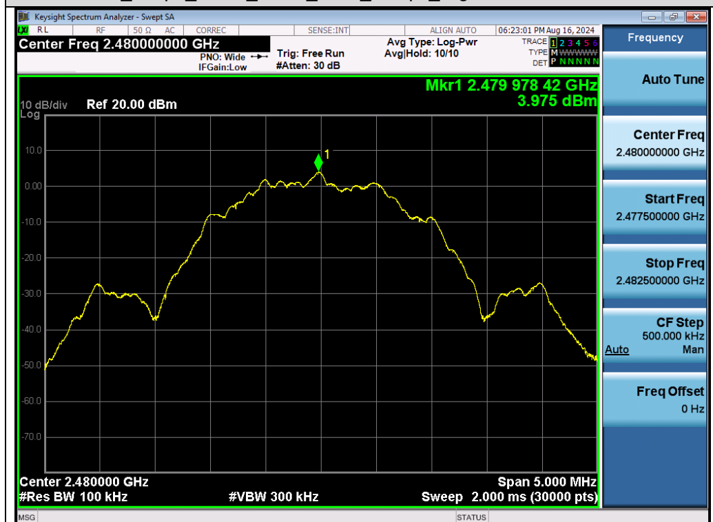
Test_Graph_LE2M_ANT1_2480_2Mbps_Reference Level
