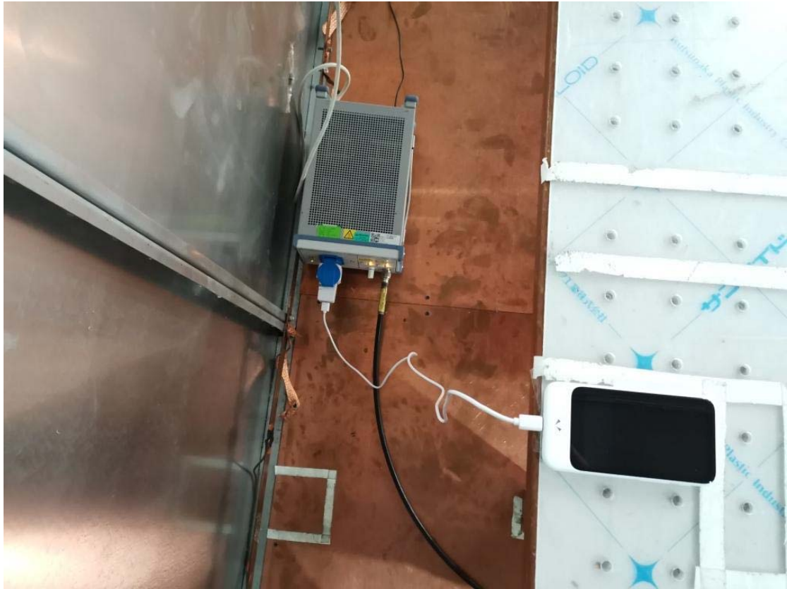
Conducted Emissions Test Setup (with charger)
