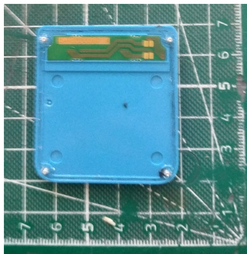
Figure 4: LEO bottom enclosure internal view
